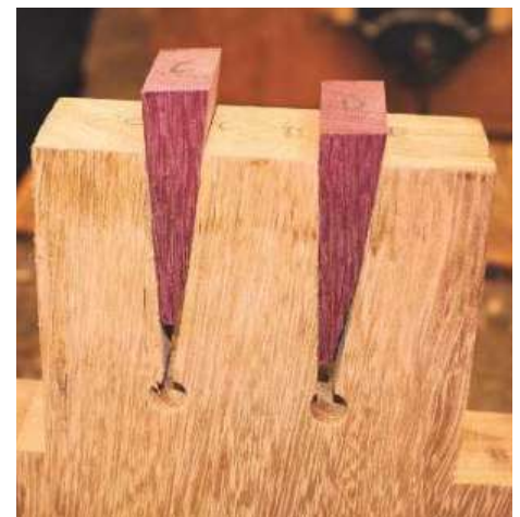
▲ Pic.5 I chose purpleheart wedges to heighten the contrast between the timbers
